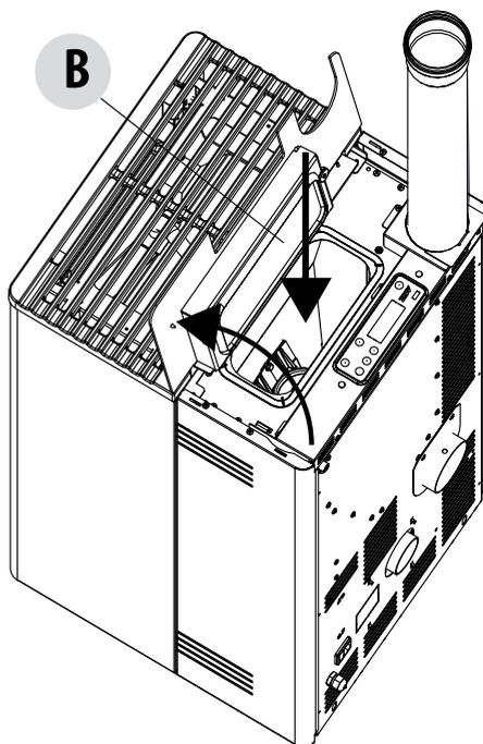
CHARGEMENT DES PELLETS SORTIE DES FUMÉES PAR
