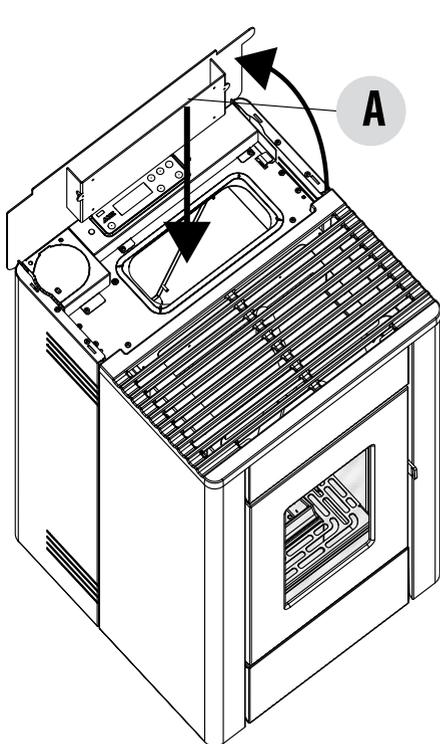
CHARGEMENT DES PELLETS SORTIE DES FUMÉES
